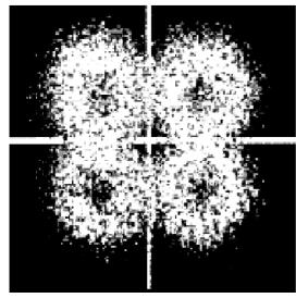
QPSK signal with intermodulation noise
